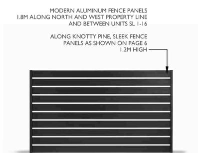
MODERN ALUMINUM FENCE PANELS 1.8M ALONG NORTH AND WEST PROPERTY LINE AND BETWEEN UNITS SL 1-16 ALONG KNOTTY PINE. SLEEK FENCE PANELS AS SHOWN ON PAGE 6 1.2M HIGH
