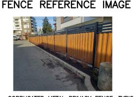
CORRUGATED METAL PRIVACY FENCE, TYPICAL FENCE HEIGHT TO BE 1.8m. CATCHMENT FENCE, IF NECESSARY TO BE 1.5m Ht. AND OMIT TOP HORIZONTAL SCREEN ELEMENTS.
