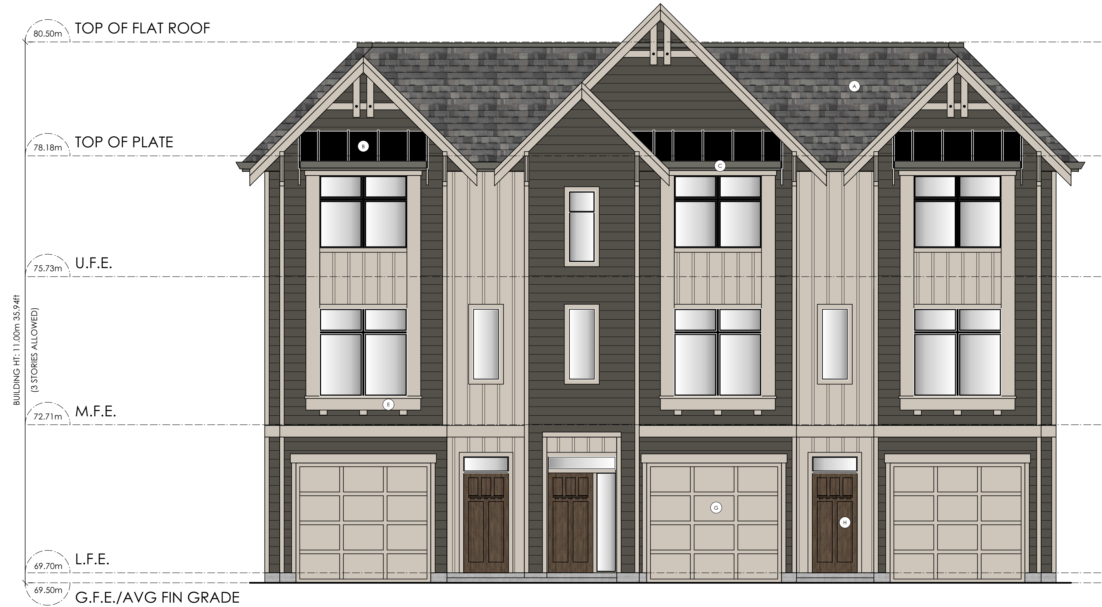
17 Type A Front Elevation (Block 6) Scale: 1/4" = 1'-0"
