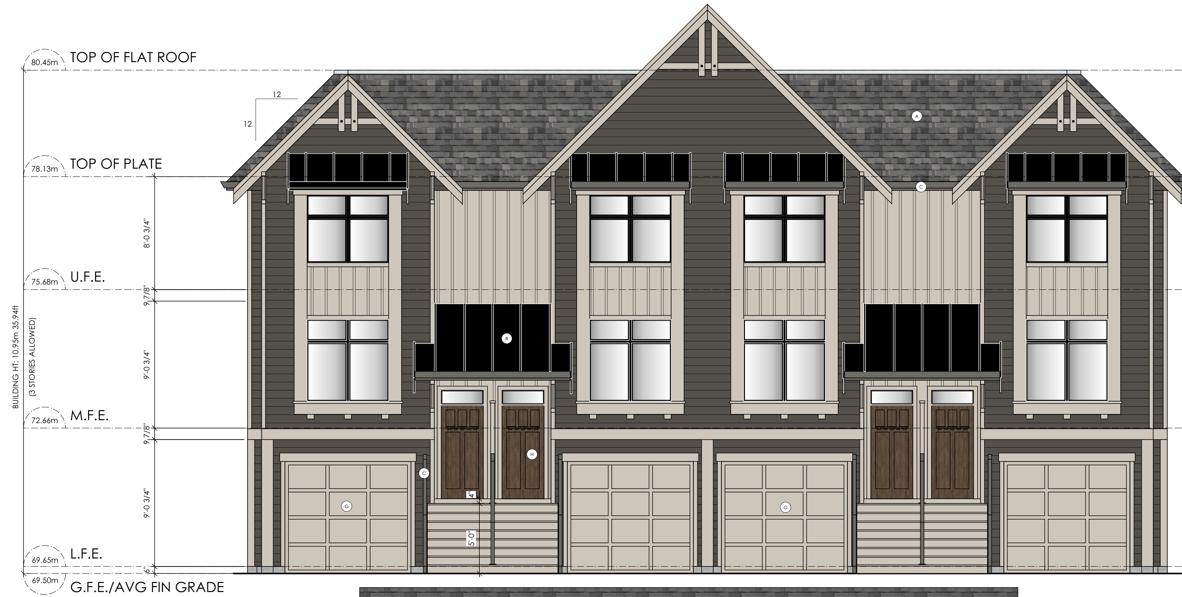
8 Type B Front Elevation (Block 5) Scale: 1/4" = 1'-0"
