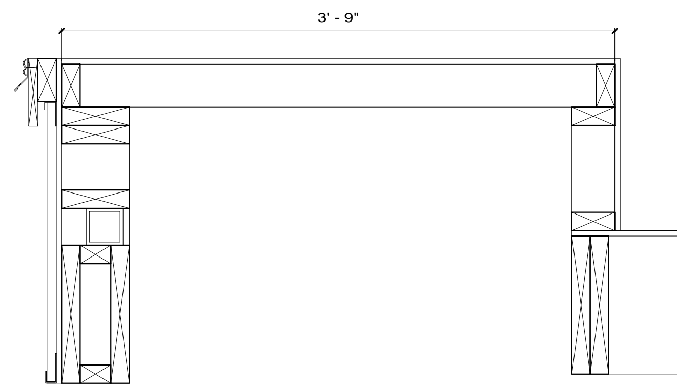
2 Bump-Up Roof Detail 1 1/2" = 1'-0"
