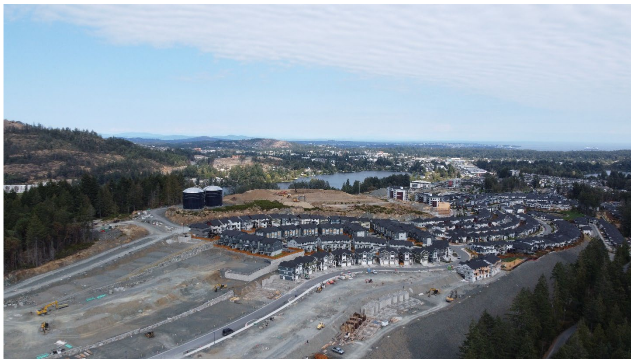
Photo 8. Hilltop water storage in the Westhills neighbourhood helps maintain pressure in the water supply system.
